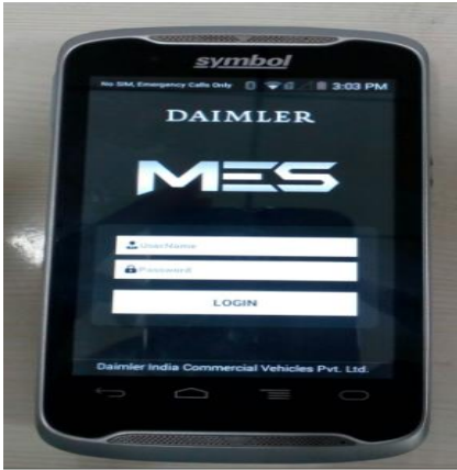
E kan ban used for material call and delivery through Mobile device (TC 55)
