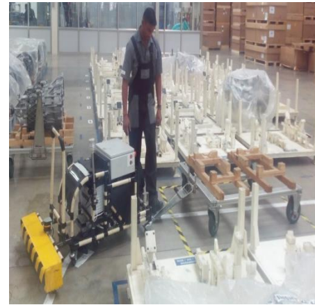
In house AGV for transferring the material with the help of magnetic lines
