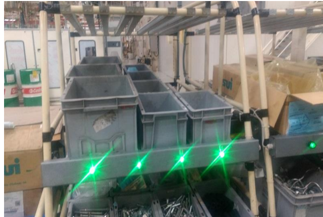
Pick to light in Daimler used for kitting preparation
